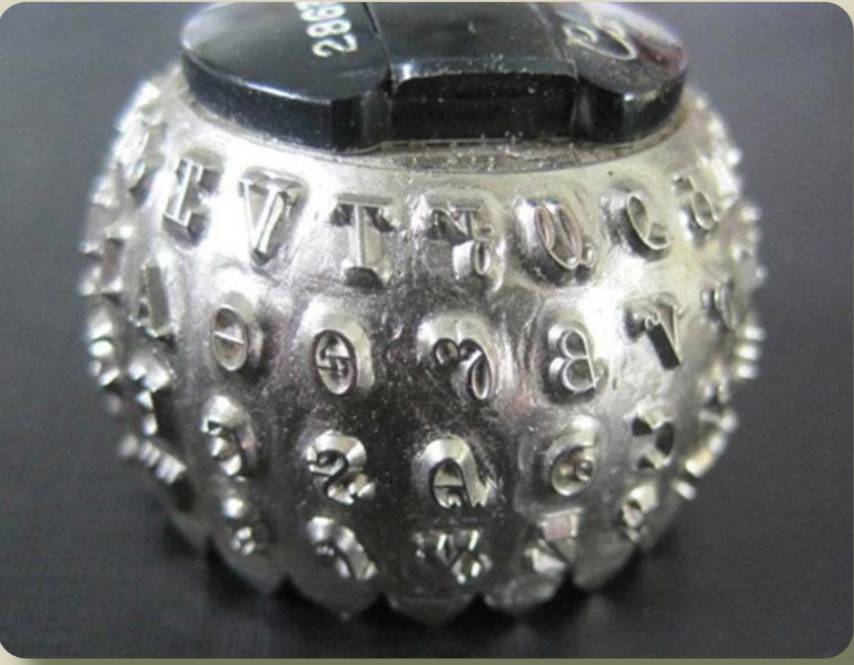
IBM Selectric Typewriter Element in Cherokee c. 1975. Image Courtesy of MaryEllen Meredith, Norman, OK, USA.
